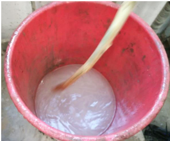
Figure 5 : Mixing NaOH Flakes in water
