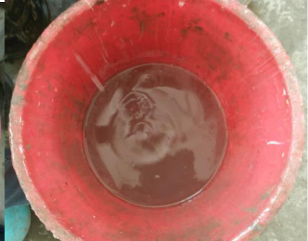
Figure 6 : Mixing NaOH Solution with Na 2 SiO 3
